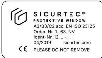
We provide all machine safety windows with a silver-coloured sticker within the machine safety window unit, or directly on the polycarbonate. The information includes our order number and ID number for traceability, the bulletproof class and European standard, and as an option, the customer's drawing or article number as well as the production date.
