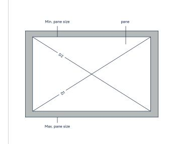
A nominally rectangular pane must be contained within a rectangle with sides having the permitted maximum and minimum dimensions.
